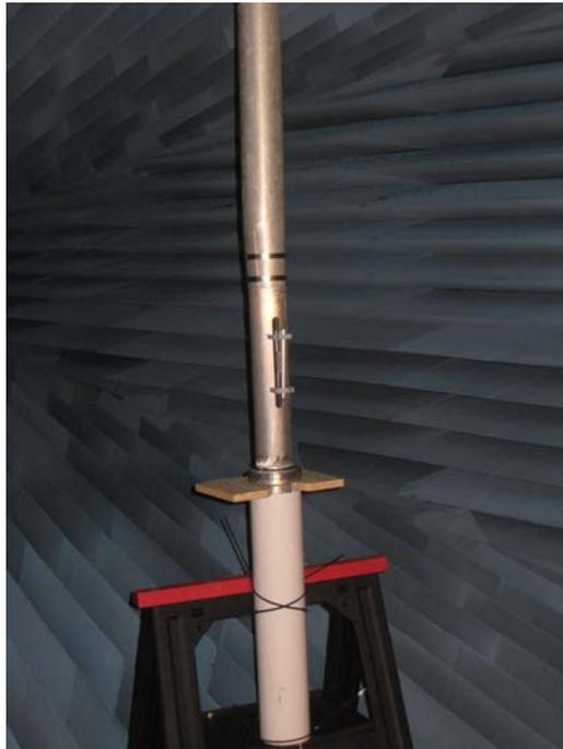
Elliptically polarized transmit antenna
