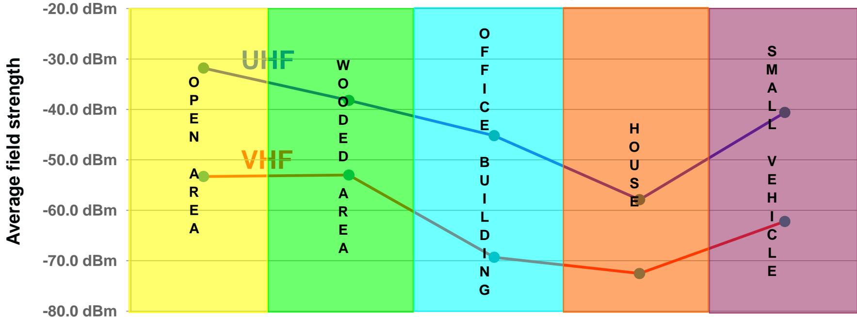
**VHF has 19.4 dB less average signal strength than UHF**
