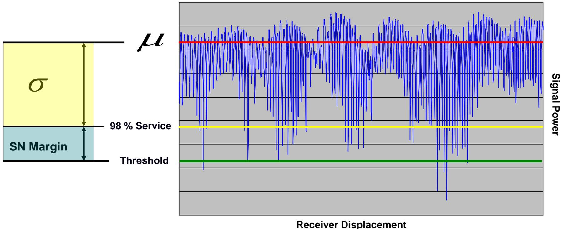
**Decreasing the variability and/or increasing the mean value of the signal strength of the received signal is exactly the same as increasing the SN margin**
