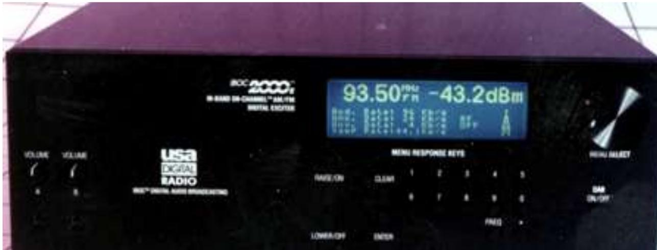
The Gen I exciter and its companion HD Radio Receiver were highly custom, single channel systems using fourteen Analog Devices SHARC Processors on a PC104 bus.
