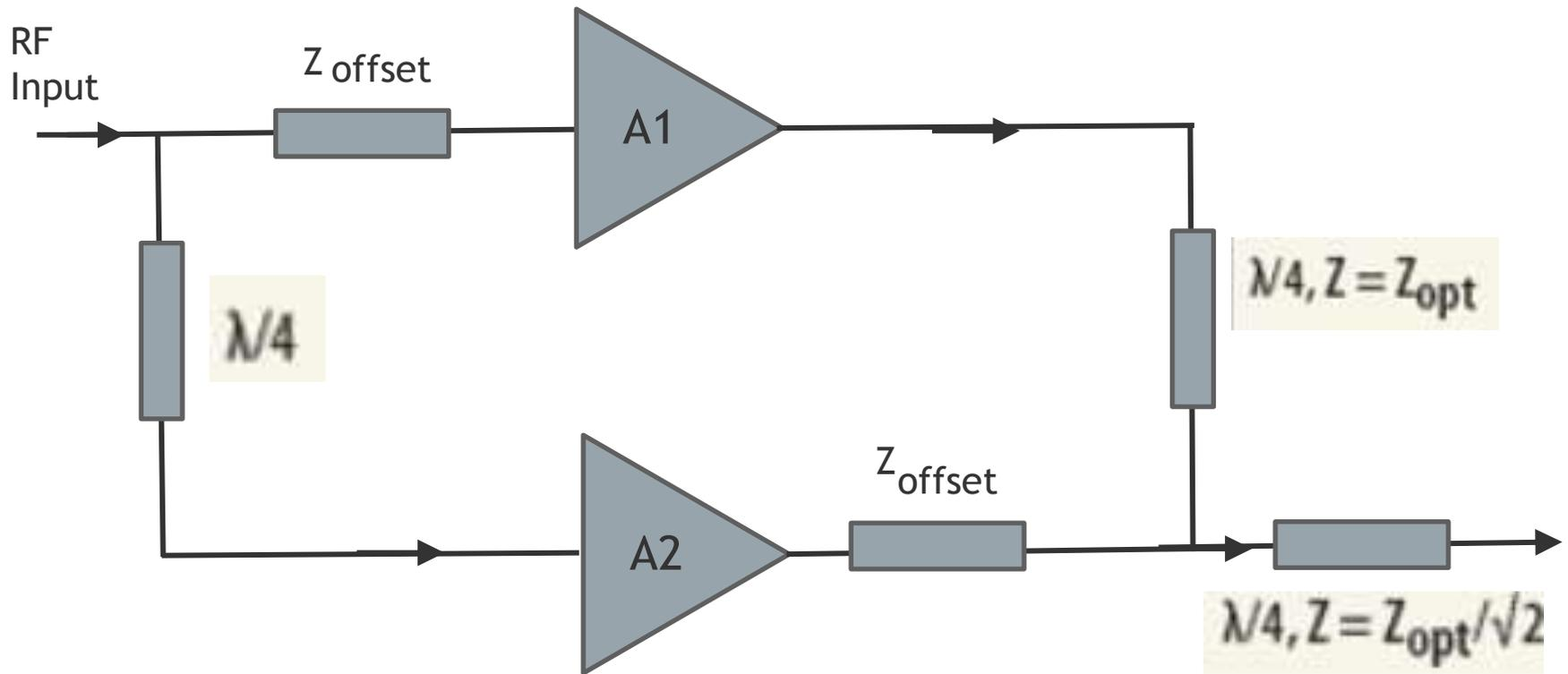
A basic **DOHERTY** architecture contains a carrier amplifier biased to operate in Class AB mode (A2) and a peaking amplifier biased to operate in Class C mode (A1).
