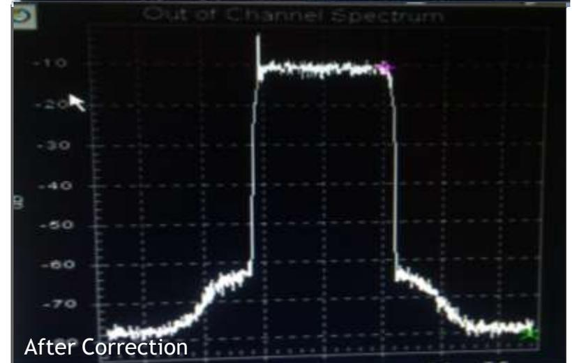
Inter-modulation decreased the in-band noise hence degrading the Signal to Noise (SNR) or Modulation Error Ratio (MER).
