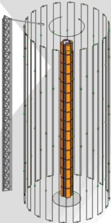
Transform data to the far field and fully characterizes the 3 dimensional radiation pattern
