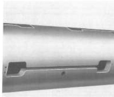
1957 RCA engineers make a breakthrough with the dog bone slot
