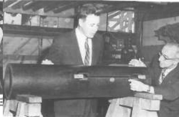
FIG. 5. An experimental short section of 18 inch diameter pipe having a pair of oppositely facing slots for a high gain Traveling Wave Antenna.
