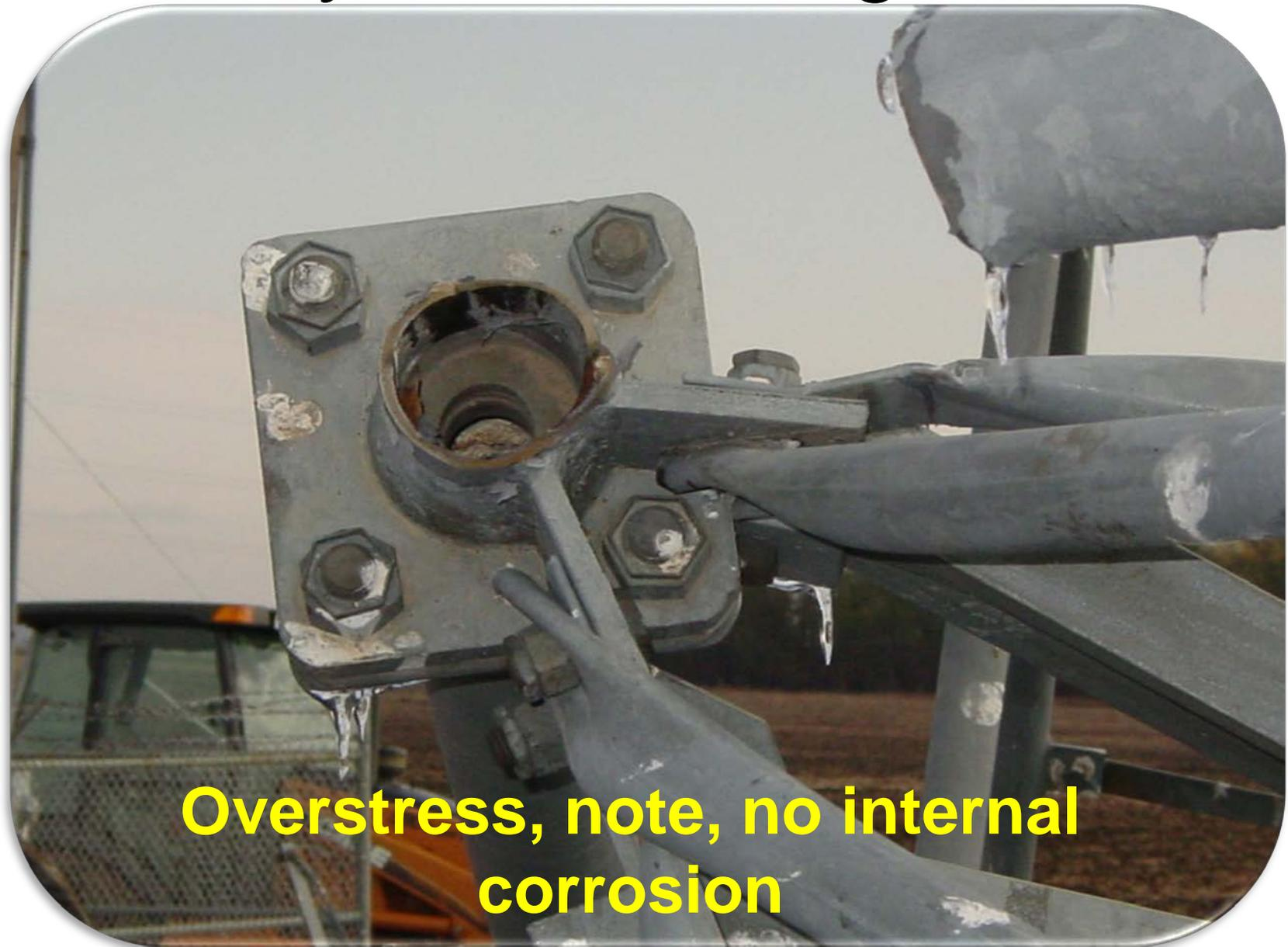
**Overstress, note, no internal corrosion**
