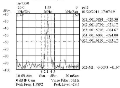
+/- 10.2 to 20 kHz Span M1: Fundamental Frequency M2: -10.2 kHz = -41.67 db M3: - 20 kHz= -55.17 db
