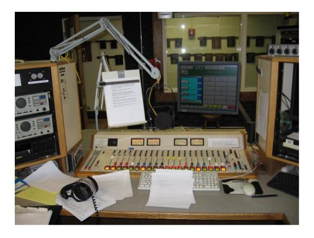
WPR Main Control Room—PR&E RMX-20 Failing switches would interrupt audio on a regular basis
