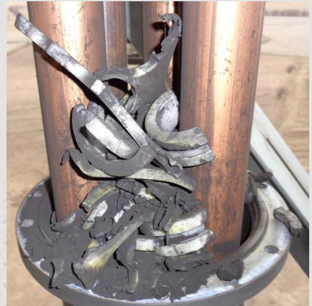
Figure 7: Collection of Melted Insulators, Inner Conductors, and Soot
