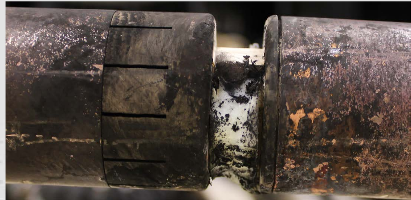
Figure 5: Melted Teflon Insulator
