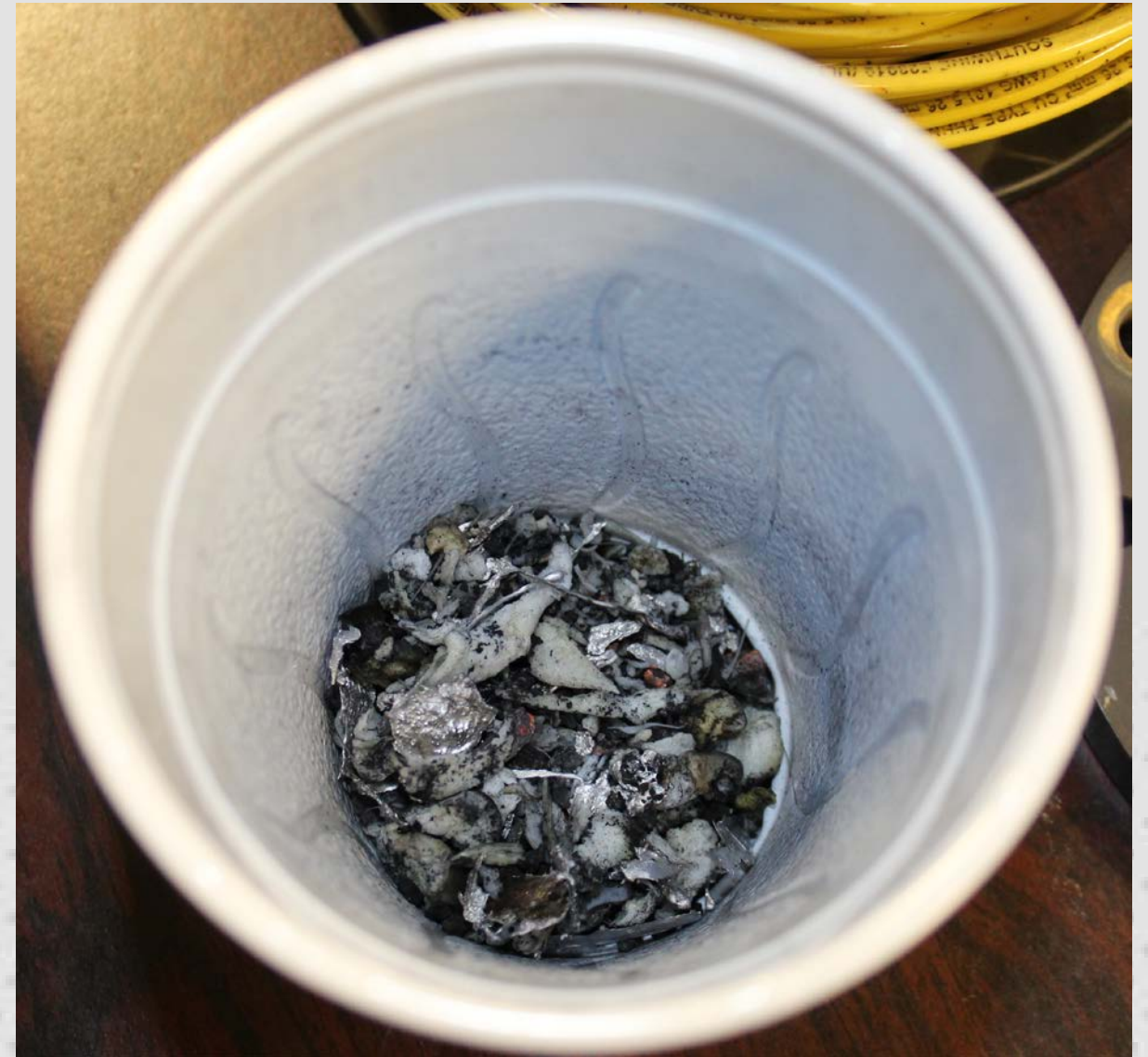
Figure 8: Debris Littered Throughout Feed System
