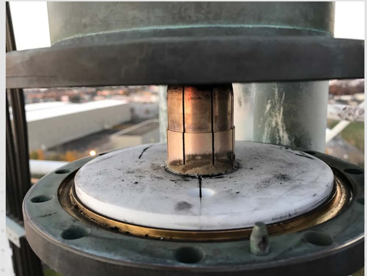
Figure 3: Carbon Build-Up On Teflon Insulator
