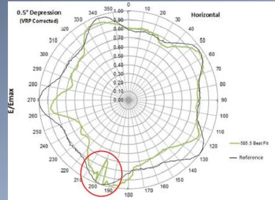
Generally seen on side-mounted antennas. A manufacturer's pre-install pattern study that accounts for the support structure, including everything metallic that passes through or near the antenna aperture can prevent most of these issues.
