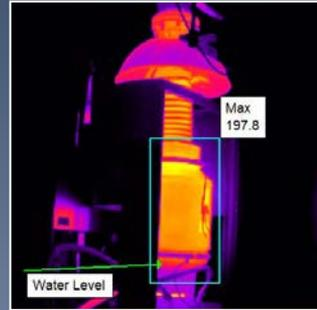
*Water cooled transmitter tubes – one is starting to get in trouble, the other IS in trouble. Look at the coolant levels.*
