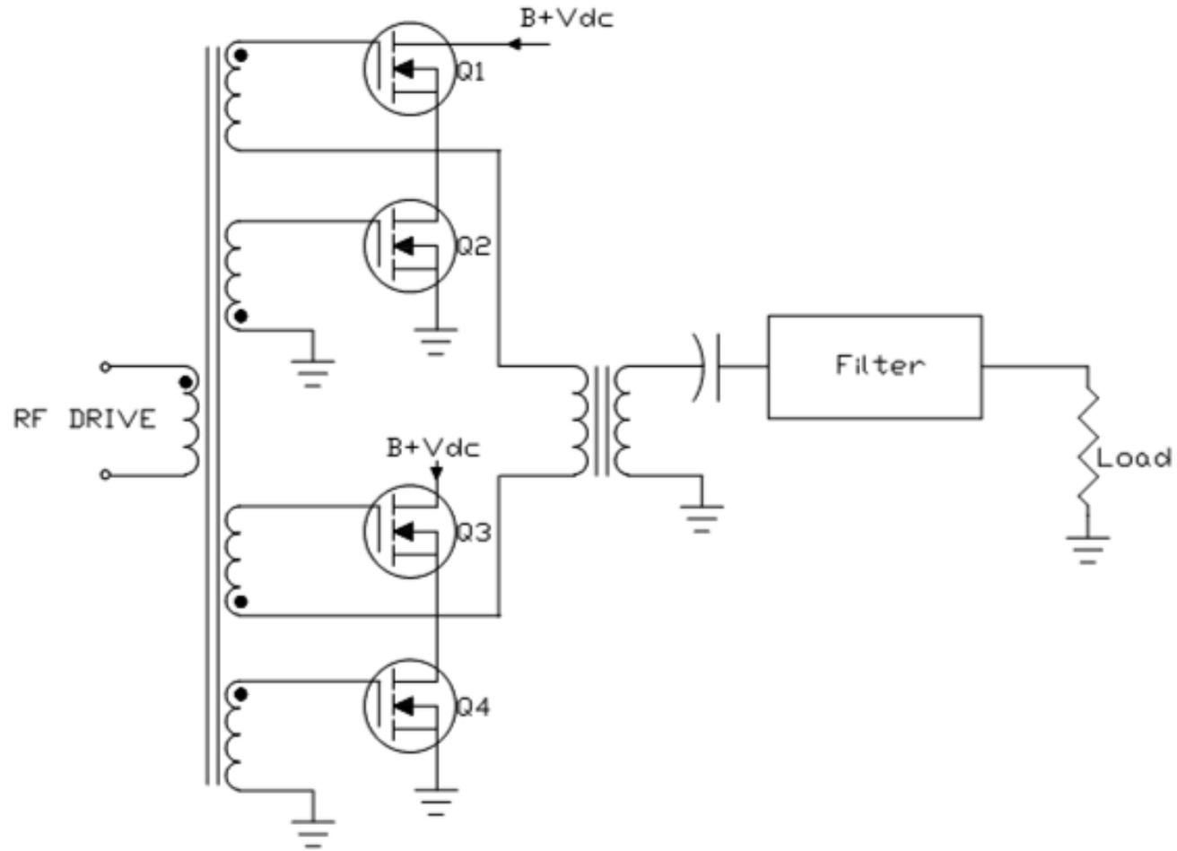
Class D Amplifier (push-pull configuration) using MOSFETs
