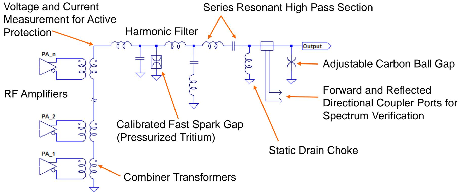
Frequency Agile: Harmonic Filter Re-Tune in a Few Hours
