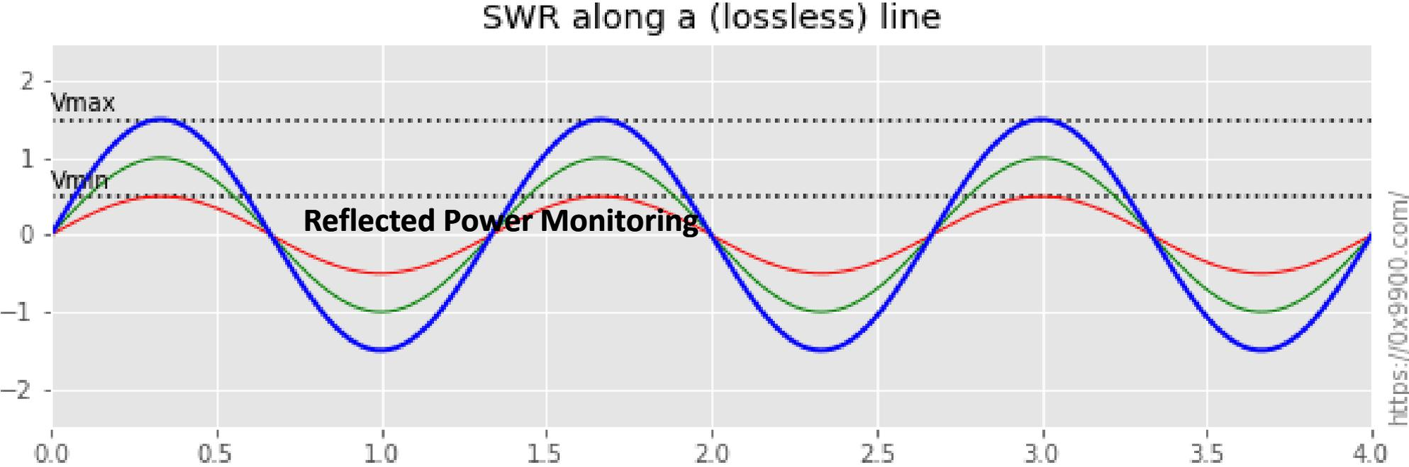
Green = Forward, incident wave    Red = Reflected wave    Blue = Composite wave
