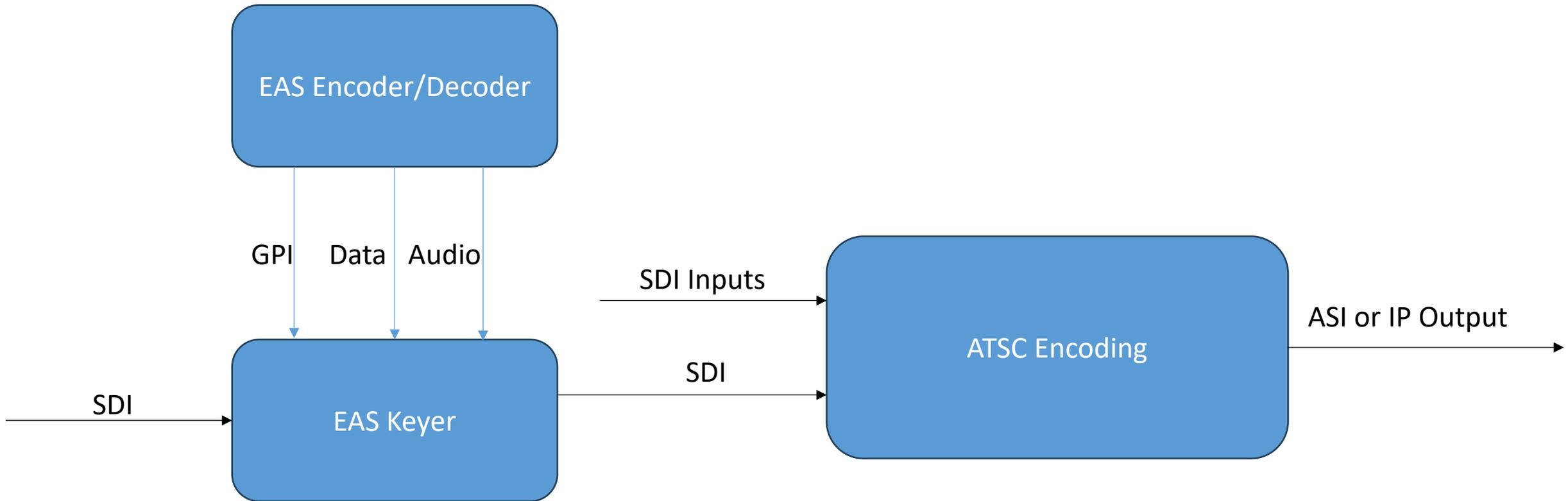
EAS Keyer required for each service, and most cards require serial data, GPI and audio from EAS unit.
