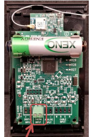
Input Terminal Block for 10K Thermistor connection
