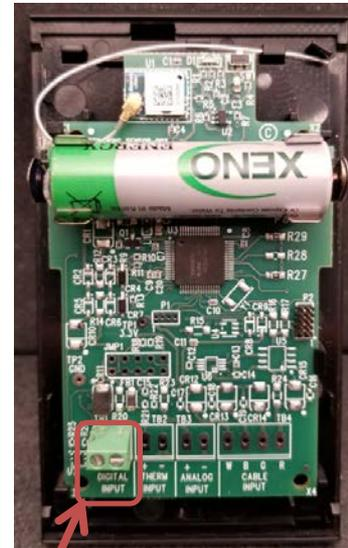
Input Terminal Block for Digital (Dry Contact) Input connection
